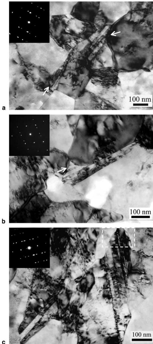
Fig. 9. Bright-field TEM micrographs of deformation twins in ultrafine grains in Cu ECAPed for: (a) 16; (b) 20 passes in the  $X$  planes and (c) 24 passes in the  $Y$  plane.
