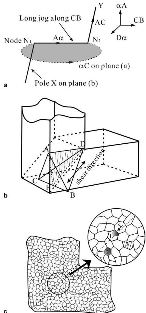
Fig. 13. (a) Pole mechanism of deformation twinning for fcc metals; (b) grain orientation for twinning in ECAP pattern; (c) twinning of ultrafine and nanometer-sized grains under ECAP shear stress.
