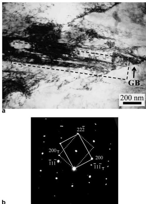
Fig. 4. TEM micrographs of deformation twins near grain boundary in CG-Cu ECAPed for one pass in the  $Y$  plane: (a) bright-field image; (b) corresponding SAD pattern with a zone axis  $[011]$ .
