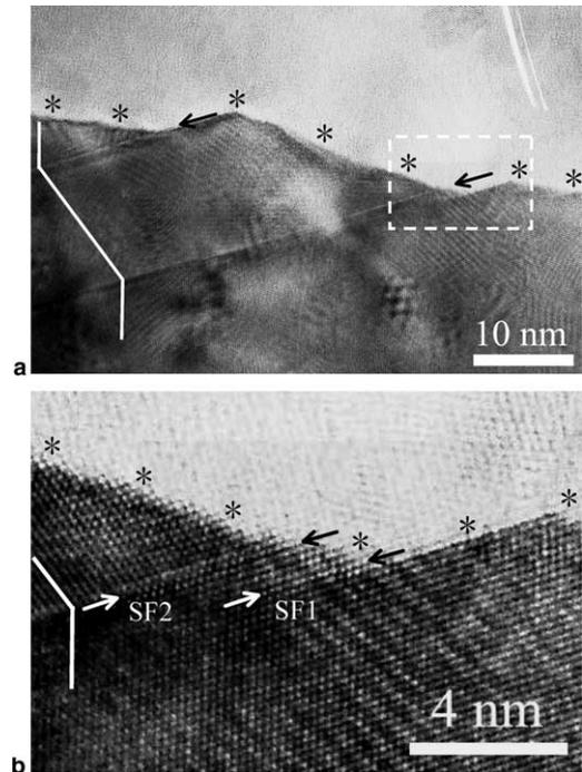
Fig. 10. [110]-direction HRTEM micrographs taken from the white frame in Fig. 9(c). (a) A curved GB segment (marked by black asterisks) with twin boundaries. The  $\{111\}$  planes that form the twin relationship among the bands are indicated by white lines. (b) An enlarged image of the white frame in (a).
