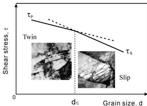
Fig. 14. Grain size dependence of the shear stress required for dislocation emission from GB of UFG- and NC-Cu.
