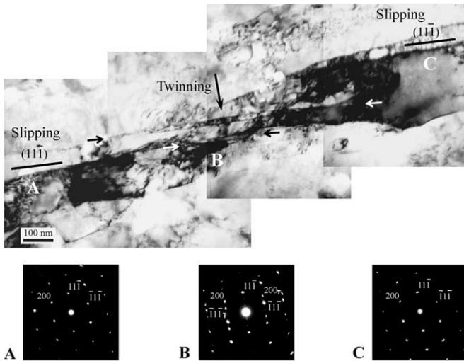
Fig. 6. TEM micrographs of deformation twins formed in a shear band. The SAD patterns with zone axis  $[011]$  taken from the regions marked with white letters A, B and C in micrograph, respectively.
