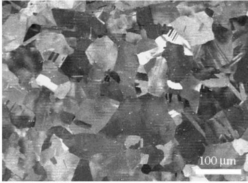
Fig. 1. SEM-electron channeling contrast micrograph of the initial CG-Cu rod.
