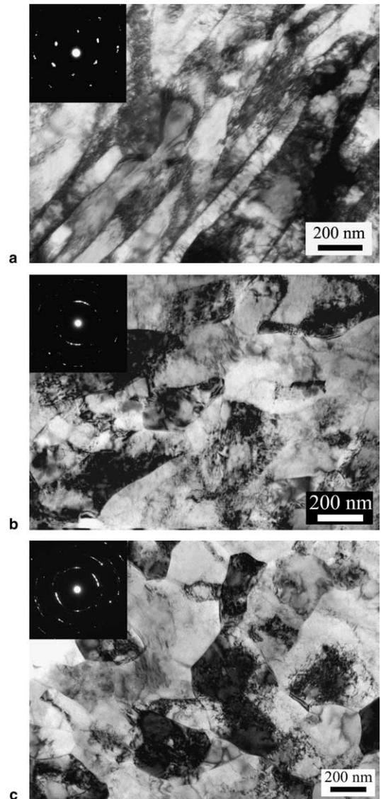
Fig. 3. Bright-field TEM micrographs of deformation microstructures of CG-Cu after ECA pressing for: (a) one pass in the  $Y$  plane; (b) eight and (c) 24 passes in the  $X$  plane.
