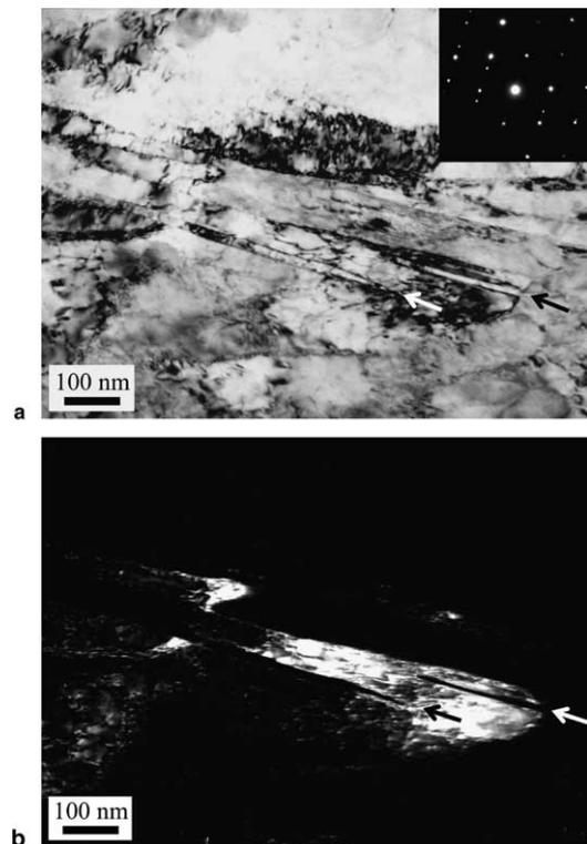
Fig. 5. TEM micrographs of deformation twins in grain interior of the sample ECAPed for one pass: (a) bright-field image; (b) dark-field image. The inset in (a) shows SAD pattern with a zone axis  $[011]$  taken from the area containing narrow bands.
