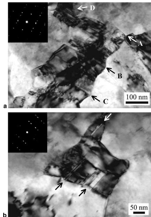
Fig. 11. Bright-field TEM micrographs of deformation twins: (a) in an ultrafine grain and a nanocrystallite; (b) in subgrains of an ultrafine grain.
