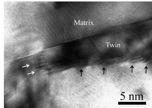
Fig. 8. HRTEM micrograph of a lenticular twin front viewed from the  $[011]$  direction.
