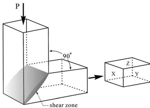
Fig. 2. Schematic illustration of ECAP process.
