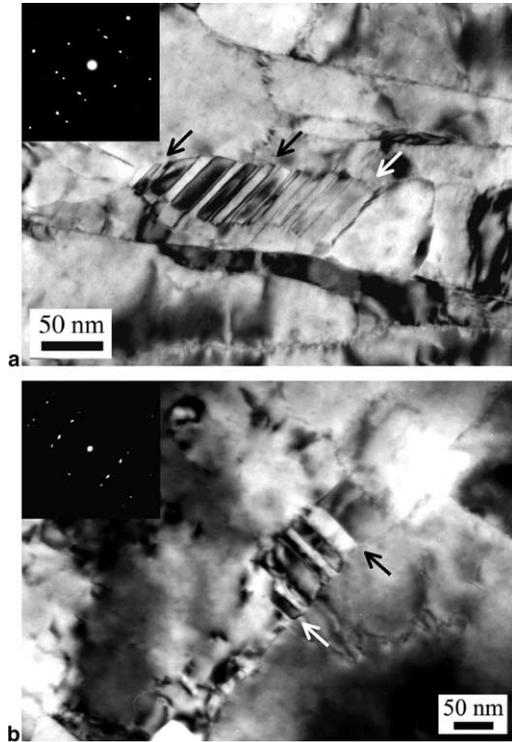
Fig. 12. Bright-field TEM micrographs of deformation twins in nanocrystallites.
