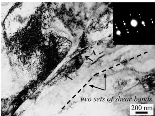
Fig. 7. TEM micrograph of deformation twins formed in the intersection of two shear bands. The inset shows SAD pattern with a zone axis  $[011]$  taken from the area as denoted by arrow A.
