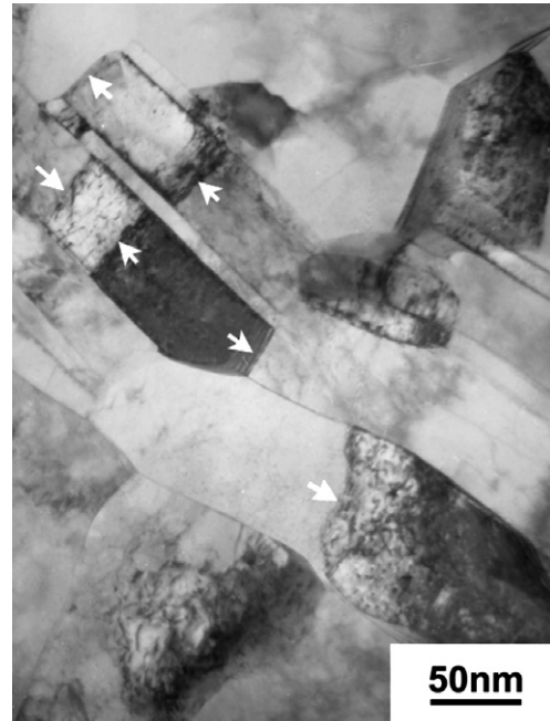
Fig. 10. A TEM image showing formation of dislocation walls (as indicated by arrows) inside twin lamellae in SMAT-30 sample.
