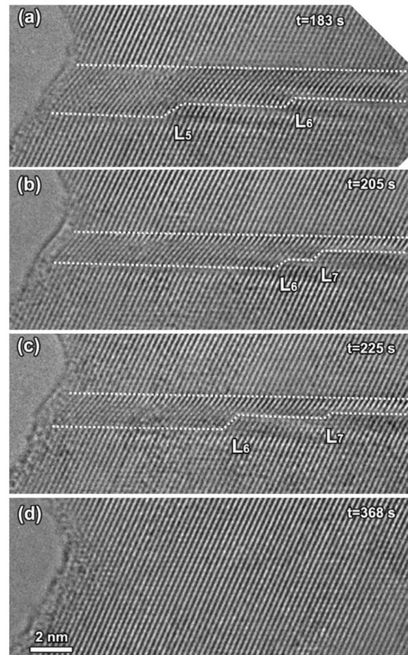
FIG. 3. A series of HRTEM images taken at different times, monitoring the detwinning process of the twin in Fig. 2. The TBs are outlined using dashed lines, and the retracting ledges on the TBs are indicated by  $L_5$ – $L_8$ . (a)  $t = 183$  s. (b)  $t = 205$  s. (c)  $t = 225$  s. (d)  $t = 368$  s.
