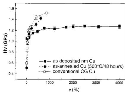
**Fig. 3.** Microhardness variation with deformation degree of cold rolling for the as-deposited nc Cu specimen, the conventional coarse-grained polycrystalline Cu, and the as-annealed coarse-grained Cu as indicated. Cracks were formed at sample edges when  $\epsilon \approx 800\%$  for the coarse-grained Cu sample.
