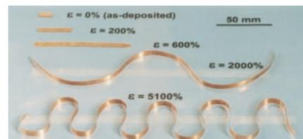
**Fig. 2.** The nc Cu specimens before and after cold rolling at room temperature with different amounts of deformation degree ( $\epsilon$ ) as indicated.
